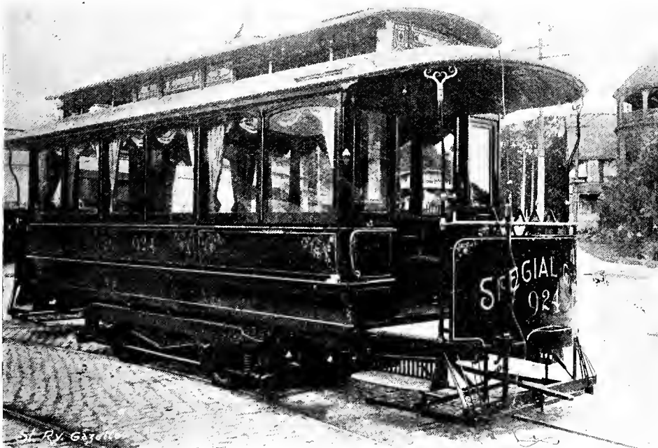
Fig. 5644. SPECIAL CLOSED ELECTRIC-MOTOR PARLOR-CAR FOR "TROLLEY PARTIES." WEST END STREET RAILWAY COMPANY, BOSTON. Length, 20 ft. Width, 7 ft. 4 ins. Seating capacity, 20 persons. Car-body built by J. M. Jones' Sons, West Troy, N. Y. West End Trucks built by the Laconia Car Company, Laconia, N. H.
